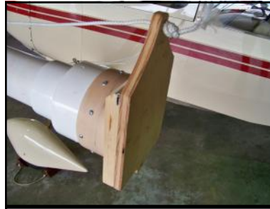
Wooden Door (in closed position) which is also connected by rope and is at the other end of the RV Slide Valve which is opened first in the dispersal.
