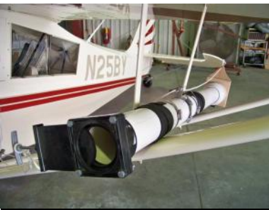
RV Slide Valve connected to the rope, which is opened to create air flow
